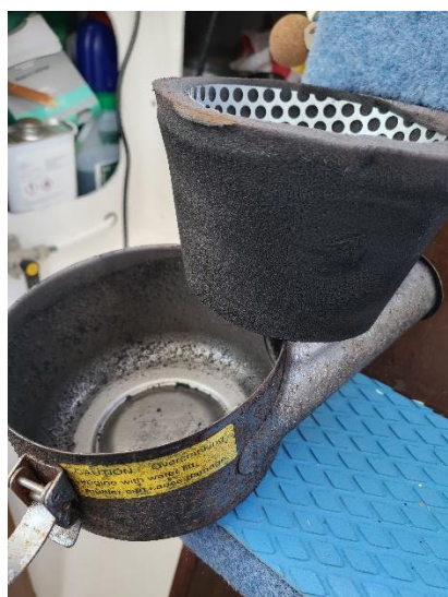
Fig 17: Clogged air filter
